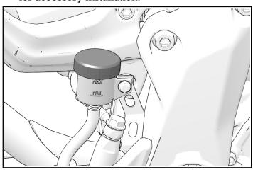
2. Hand-tighten accessory reservoir cover. Ensure retained seal is between cover and reservoir.
