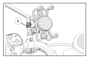
3. Widen X-Grip® to fit mobile device and stretch each corner of tether over corners of mobile device.
