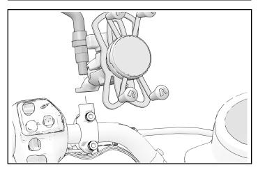
2. Tighten mirror jam nut (A).
