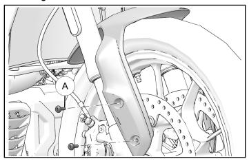
2. Align RH fork guard ① with front mudguard. Loosely install top fastener ④ and compression limiter ⑥ before securing bottom. Loosely install bottom with bottom fastener ③ and compression limiter ⑤.
