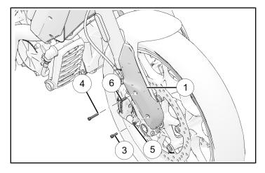
3. Remove and discard two screws (A) from mudguard.
