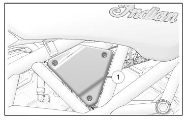
2. Install accessory V-cover ② with three retained V-cover fasteners.
