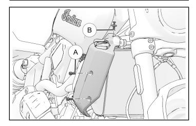
2. Remove two radiator cover fasteners (A) and one push-pin (B) from radiator cover.
