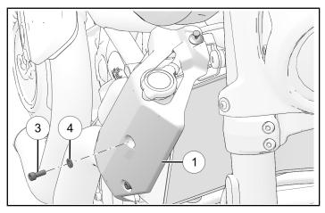
2. Install left-hand radiator guard ② with two fasteners ③ and two washers ④. Secure top of radiator guard with retained push-pin rivet.
