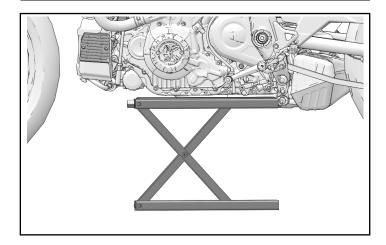
1. Secure motorcycle in an upright position with tie-down straps and platform jack positioned beneath engine cases.
