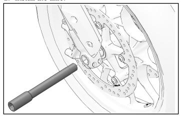
3. Make sure wheel speed sensor is installed between left fork and wheel.
