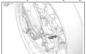
3. Support wheel and remove axle.
