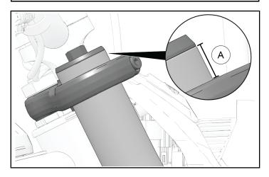
3. Torque lower triple clamp fasteners to specification.
