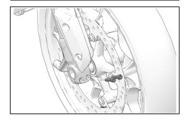
6. Install front wheel speed sensor harness to left fork.
