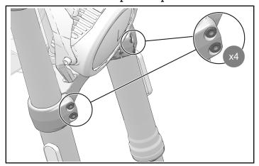
3. Carefully move fork assemblies downward and out of triple clamps.
