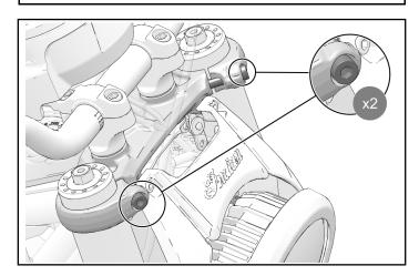
5. Torque lower triple clamp fasteners to specification a second time.
