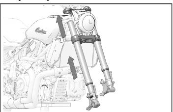
2. Continue to install fork assembly into upper triple clamp. Leave **11 mm** between top triple clamp and adjustment dial, as shown.
