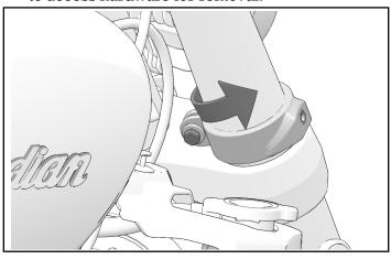
2. Remove one fastener, two bushings, and one nut to remove headlight cowl mount.
