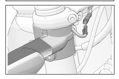
Remove and keep one screw and one washer from turn signal mount. Remove turn signal assembly from motorcycle.
