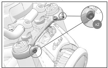
2. Loosen four lower triple clamp fasteners.
