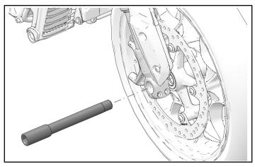
Wheel speed sensor will fall out when axel and wheel are removed.
