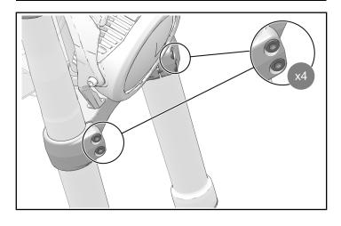
4. Torque upper triple clamp fasteners to specification.
