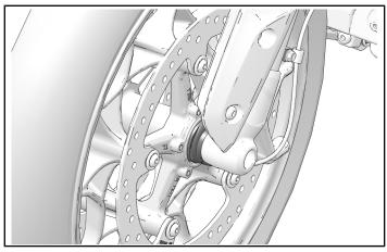
4. Torque axle to specification.
