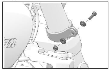
2. Turn headlight cowl mount to installed position and hand tighten fastener.
