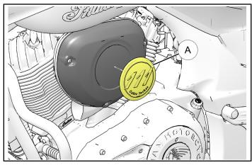
2. Remove any extra adhesive from surface. Clean surface with Isopropyl Alcohol.
