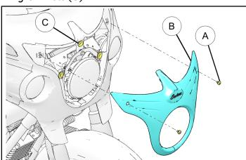
2. Insert the headlight bezel ① by inserting bezel features into the rubber grommets (C) in the fairing. Install two M6 socket head screws ② and torque to specification.
