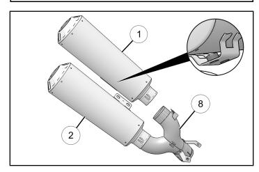
Secure mufflers to exhaust pipe with two springs
