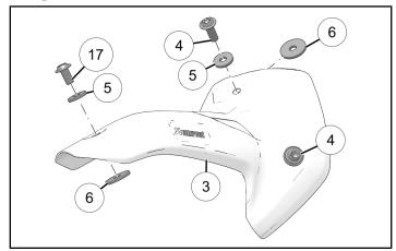
9. Install heat shield ③ onto exhaust pipe. Ensure spacers are aligned with clip-nuts underneath heat shield.
