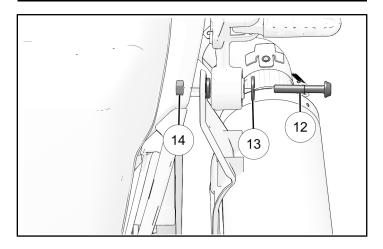
Exhaust mount with integrated spacer: Remove muffler isolator fastener <sup>(1)</sup> previously used in this section. Reinstall with one washer <sup>(3)</sup>, one retained spacer (if applicable), and integrated spacer.
