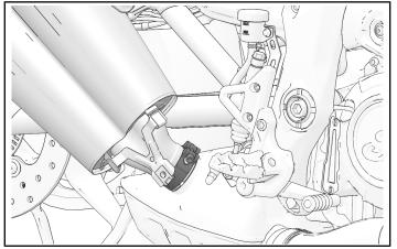
3. Remove muffler isolator fastener. Retain loose spacer (if applicable) between muffler assembly and passenger foot peg mount.
