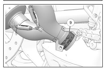
4. Install exhaust mount to passenger foot peg.
