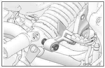
2. Slide exhaust pipe clamp (9) onto base of exhaust pipe and place exhaust pipe onto exhaust resonator.
