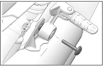
4. Remove muffler from resonator.
