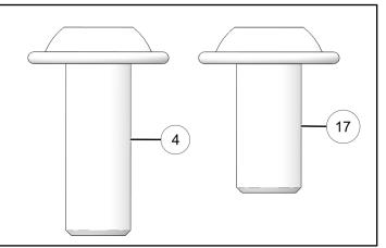
8. Pass heat shield fasteners ④ and ⑦ through three washers ⑤, heat shield ③, and three spacers ⑥.
