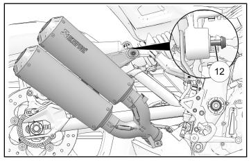
• Exhaust mount with integrated spacer: Align exhaust assembly behind passenger foot peg and pass isolator fastener (1) through foot peg mount and loosely thread fastener into integrated spacer.
