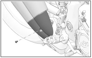
2. Loosen exhaust clamp retaining muffler to exhaust resonator.
