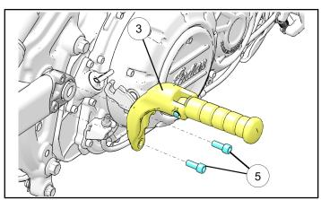
2. If desired, install passenger foot guard ④ onto right hand footpeg support ③. Mount passenger foot guard using two fasteners ⑥. Torque fasteners ⑥ to specification.
