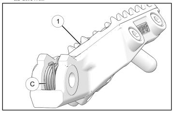
2. Place foot peg ① into foot peg mount and pass retained pin ⑧ through mount and foot peg ①. Ensure spring-end ⓒ is fitted in foot peg mount cavity.
