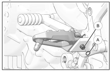
2. Remove and retain one pin (B) and one foot peg spring (C) to remove foot peg.
