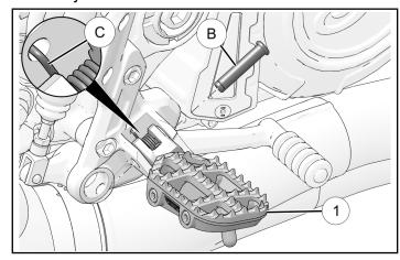
3. Secure pin (B) with retaining ring (4).
