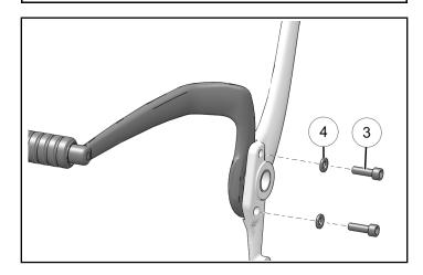
Reinstall shifter assembly onto pivot shaft. Reinstall pivot shaft and wave washer to floorboard assembly.
