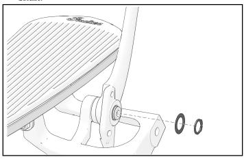
2. Remove shifter, pivot shaft, and wave washer from assembly.
