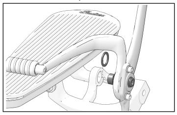
5. Secure shifter to floorboard assembly with washer and retaining ring.
