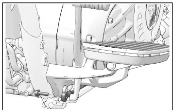
2. Remove two floorboard fasteners and remove floorboard assembly from motorcycle frame.
