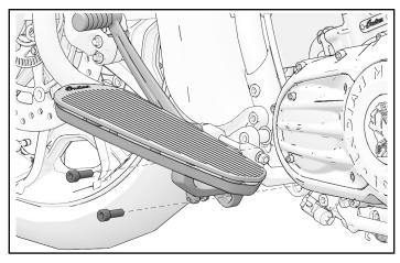
2. Install shift rod to shifter with front shift rod fastener.
