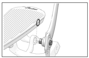
3. Align heel shifter with toe shifter and install with two fasteners ③ and two washers ④.
