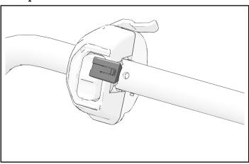
10. Slide RH switch cube off handlebar and gently set aside.
