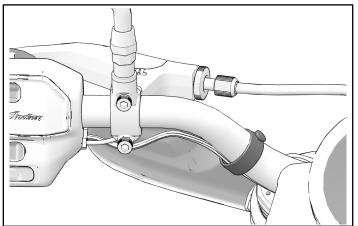
2. Use small pick to push in connector tabs to disconnect LH control harness and clutch..
