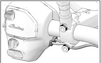
3. Remove and retain two screws (B) to separate side-mirror perch and clutch lever. Gently let clutch hang and place mirror perch aside.
