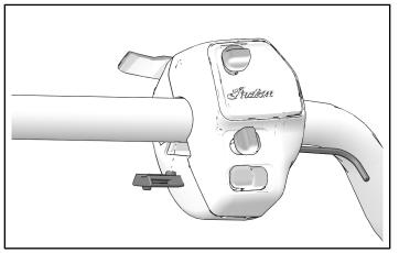
6. Slide LH switch cube off handlebar and gently set aside.
