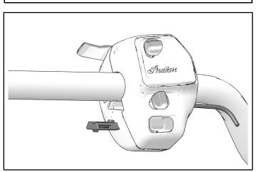
2. Loosely install mirror perch to clutch lever with two retained screws (B). Ensure mirror/clutch lever positioning is at desired position before torquing hardware.
