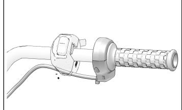
4. Loosely install handlebar with two riser caps and four retained screws  $\mathbb{C}$ .
