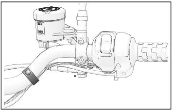
2. Use small pick to push in connector tabs and disconnect RH controls.
