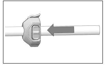
2. Place mounting clip into hole and slide RH switch cube into installed-position until switch cube snaps into place on mounting clip.
