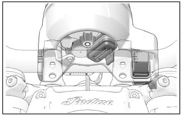
3. Install instrument cluster with two retained screws (A) and two retained washers (B).
