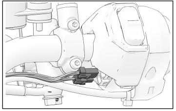
9. Secure RH switch cube harness to handlebar with retained rubber cable tie.
