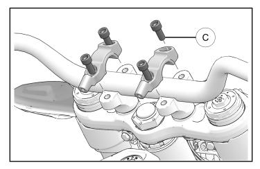
5. Adjust handlebar to 0 index. Torque screws, installed in previous step.
