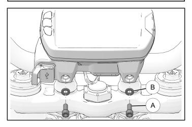
Disconnect electrical harness connector and two USB connectors before removing Ride Command<sup>™</sup> from handlebar.
