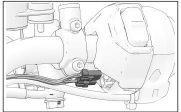
3. Loosen, but DO NOT remove, screw (A) from electronic throttle control (ETC).
