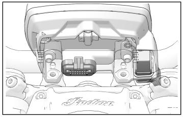
Remove and retain two bushings C and two rubber washers D from rear of Ride Command<sup>™</sup> assembly.
