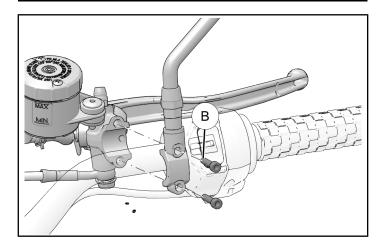
5. Remove and retain four screws C and two clamps to remove handlebar.
