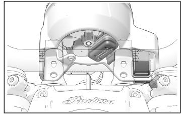
3. Remove and retain two bushings (C) and two rubber washers (D) from rear of instrument cluster.
