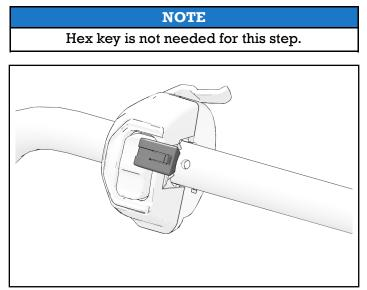
3. Slide ETC onto handlebar.
