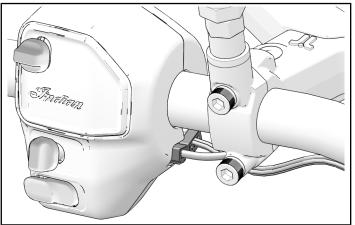
4. Secure LH switch cube harness to handlebar with retained rubber cable tie.
