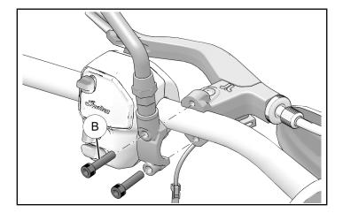
3. Reconnect clutch and harness connectors to LH switch cube.
