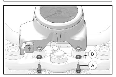
2. Disconnect electrical harness connector and two USB connectors before removing instrument cluster from handlebar.
