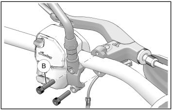
4. Use 2 mm hex key to disengage mounting clip, located beneath LH switch cube. Simultaneously, slide LH switch cube towards center of handlebar
