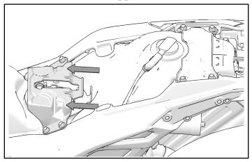
3. Slide seat into seat support bracket and into front mounting bracket.
