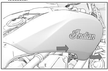
5. Pull each cover directly upward and free of alignment tabs.
