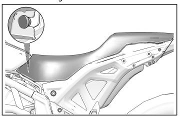
4. Secure rear of seat with two retained seat fasteners (8).
