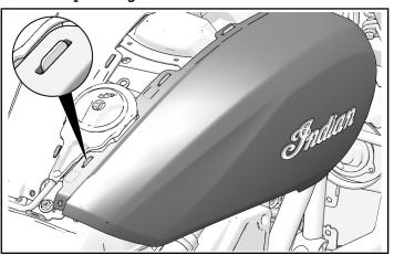
4. Firmly push lower tank cover into grommets. Ensure both tank cover rivets are firmly seated and grommet has not been pushed through bracket.
