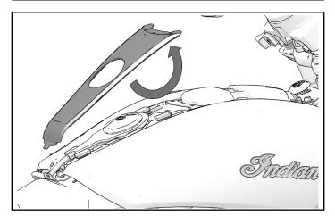
3. Remove and retain two tank cover fasteners © from rear-end of tank covers.
