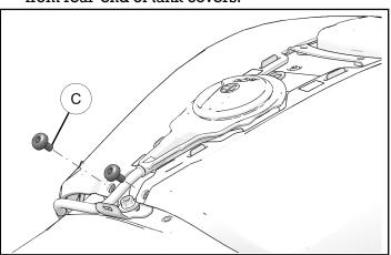
Pull bottom of each tank cover outward to disengage plastic rivets at two marked locations.
