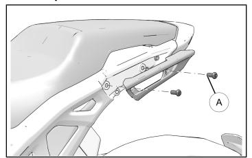
2. Remove and retain one seat fastener ® from each side of motorcycle frame.
