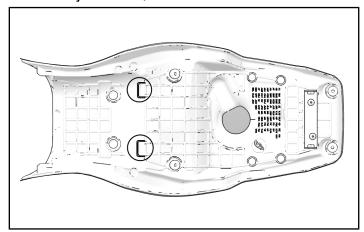
2. Tabs, identified in step 1 of this section, will slide beneath seat support bracket.
