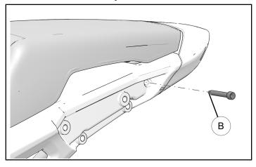
3. Slide seat back-and-up, to ensure seat slides out of mounts, to remove from motorcycle.
