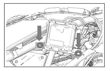
3. Place each tank cover on alignment bracket. Ensure each alignment tab is seated within corresponding tank cover hole.
