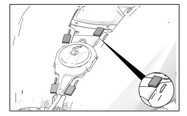
7. Place tab of center console into bottom bracket and flip down into installed position. Press firmly at adhesive pad locations to ensure each pad sticks to tank cover.
