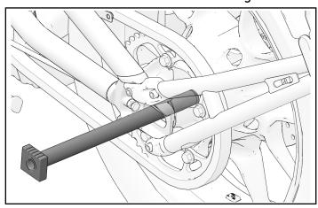
7. Remove rear wheel assembly by sliding it to rear of motorcycle.
