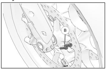
4. Support wheel and remove axle. Spacer is loosely retained by dust seals, but may fall out after wheel has been removed.
