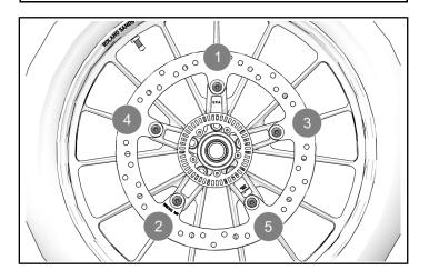
3. Install ABS tone ring with five retained fasteners
