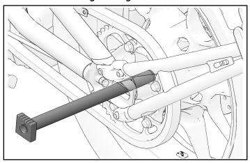
3. Move wheel rearward to gain access to install wheel speed sensor mounting bolt (E) and sensor.
