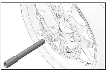
3. Cycle front suspension. Tighten axle pinch bolts
