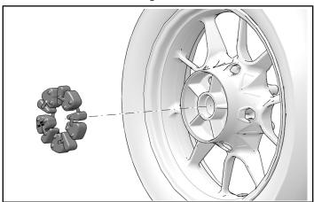
2. Install sprocket assembly onto wheel hub. Make sure drive damper properly engages sprocket assembly.
