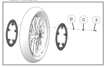
2. Torque brake disc fasteners to specification in star pattern.
