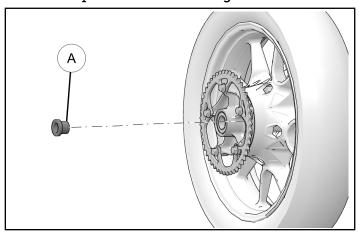
2. Remove driven sprocket assembly from drive damper.
