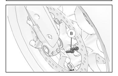
4. Install front wheel speed sensor with fastener (A).
