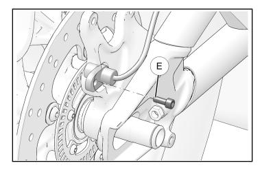
6. Loosely install nut onto axle and tap nut to start pushing axle out other side. Remove nut, slightly lift wheel and remove axle from swingarm.
