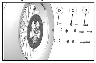
2. Torque brake disc fasteners to specification in star pattern.
