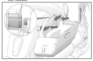
Push the latch cams downward to lock the saddlebag onto the vehicle. Resistance must be felt when locking the latch cam to ensure a secure mount.
