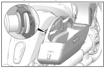
3. With the latch cams held horizontally, guide the rubber bushings into the mounting spools on the vehicle.
