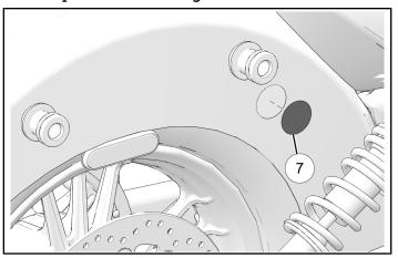
3. Note location of bumper, remove backing from protective film and apply film to fender. Repeat on opposite side.
