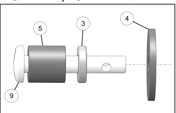
2. Insert anchor pin assembly (9) into mounting hole of saddlebag and slide cam latch (6) onto end of pin.
