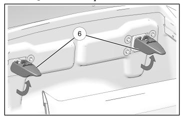
2. Hook saddlebag brackets to spools and align rubber grommets with spools as shown.
