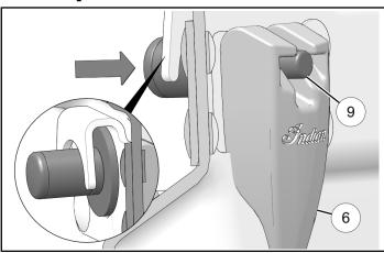
3. Hold latch (6) in place and compress pin (9). Insert dowel pin (8) into hole in anchor pin (9).
