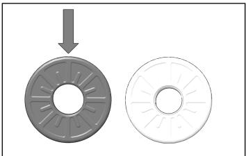
2. Thinly coat inside of RH grip ② with isopropyl alcohol to help reduce friction during installation. Install by twisting grip back-and-forth until fully seated on handlebar.
