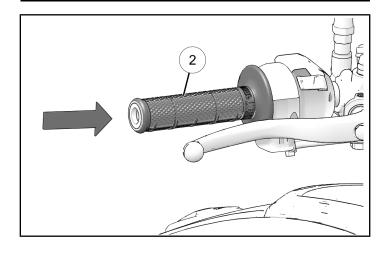
3. Partially thread bar end fastener (A) into wedge anchor assembly. Slide wedge anchor into handlebar tube until bar end is flush against handlebar tube.
