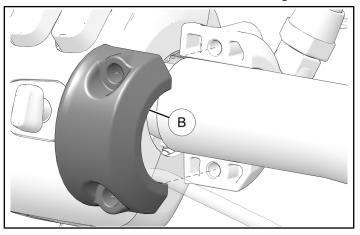
3. Thread RAM<sup>®</sup> ball mount ① into RAM<sup>®</sup> clutch mount ② as shown.
