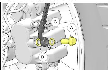
2. Remove and discard banjo bolt ① and two seals ② from upper end of front brake line ③.
