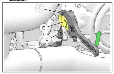
4. Free clutch cable ① from motorcycle up to clutch handle ⑥ and remove stock clutch cable and discard.
