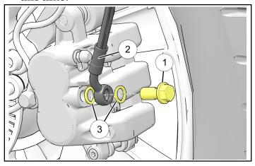
3. Install new front brake hose end ② to front brake lever using one new banjo bolt ① and two new seals ③. Do not torque banjo bolt at this time.
