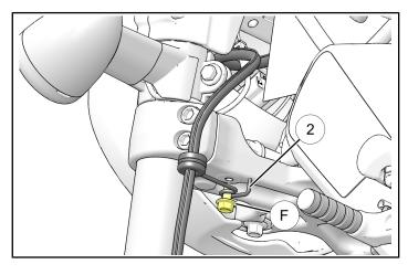
5. Ensure brake lines are routed properly and torque new banjo bolts ① to specification.
