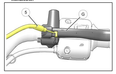
3. Loosen jam nut (H) on new clutch cable (5), apply multi-purpose grease to cable and install cable end into mounting bracket.
