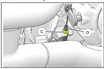
3. Using a wrench, turn clutch arm (E) to release tension on cable (D). Remove cable end (F) from clutch arm. Remove clutch cable (D) from bracket.
