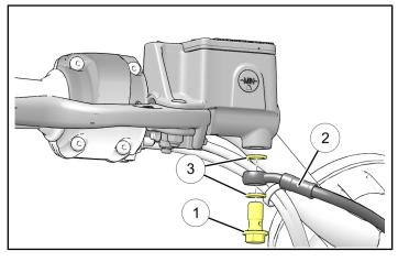
4. Install wire bracket for new brake line ② onto loosened bolt ⑤. Adjust brake line to original location and torque screw ⑥ to specification.
