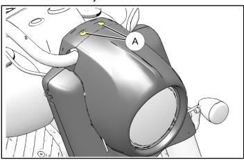
3. Remove and retain two fasteners ® from each side of nacelle assembly. Disconnect turn signals © and light bar bracket (if installed-not shown) and set aside to prevent damage.
