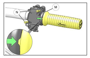
6. Loosely reinstall clutch handle assembly (f) using two retained screws (g). Reinstall clutch wire connector (1) to switch assembly (M).
