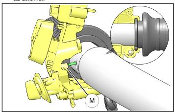
5. Quickly reinstall outer switch assembly (M) with two retained screws (N). Switch assembly notch should fit over tab on grip flange as shown with arrow. Rotate and adjust grip to fit properly. Torque screws to specification.
