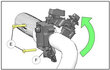
4. Slide RH throttle tube/grip from handlebar.
