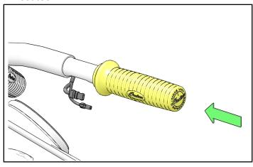
4. Quickly orient switch housing (M) with pin in rear half of housing and hole in bar as shown. Ensure to line up slots on LH Grip to switch housing (M) as shown.
