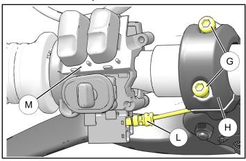
4. Remove and retain two screws (N) from inner half of LH switch (M). Rotate switch side upward and remove entire assembly. Disconnect wires from switch cube (M).
