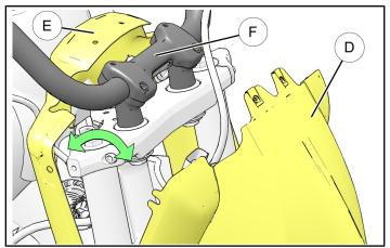
5. Loosen front handlebar clamp fasteners (a) (Do not remove screws) and rotate handlebar up until rear portion of nacelle (a) can be removed.
