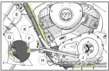
6. Remove and retain screw ① and P-clamp M.
