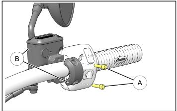
2. Remove and retain two screws © from RH switch cube cover ① and separate halves of cover.
