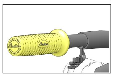
2. Orient throttle housing (f) with pin in rear half of housing and hole in bar as shown. Ensure to line up slots in throttle tube to throttle housing (f).
