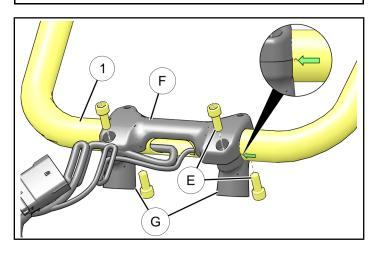
3. Carefully slide accessory handlebar ① and riser assembly into triple clamp frame D. Ensure rubber inserts B are installed. Install two retained bolts A and washers C (removed in step 1. of previous section), Torque to specification. Route handlebar wiring towards front.
