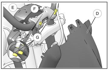
6. Disconnect auxiliary light switch (if equipped) and remove rear portion of nacelle.
