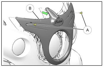
3. Remove and retain three fasteners © and withdraw head light assembly ® far enough to disconnect electrical connector. Remove head light assembly and set aside.
