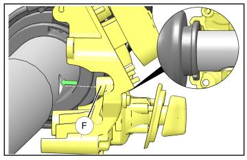
3. Close throttle housing **(F)** and reinstall two screws **(E)**. Torque screws to specification.
