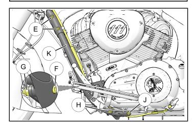
3. Install retained screw 1 and P-clamp M. Torque screw to specification.
