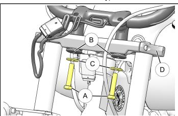
2. Remove and retain two front and two rear cap screws ©. Remove cap © and risers © from handlebar.
