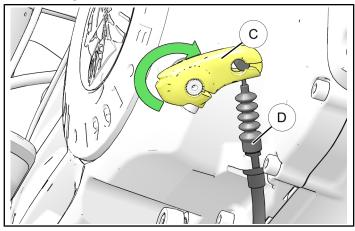
3. Withdraw clutch cable ① from mounting boss located on primary cover.
