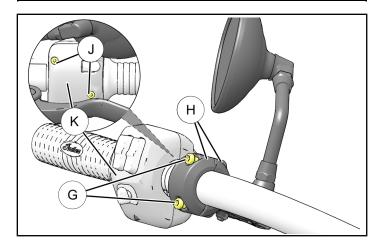
2. Remove and retain two screws ① from LH switch cube cover ⑥ and separate halves of cover.
