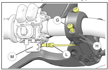
7. Reinstall LH switch cube cover (k) using two retained screws (J). Ensure that all wiring is held within switch cube (k) and is not pinched. Ensure clutch wire is not pinched by housing. Torque screws to specification.
