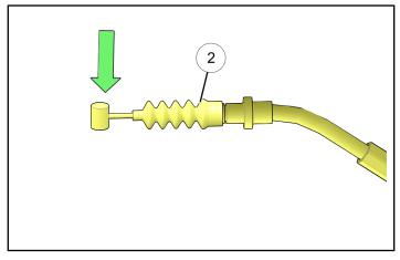
9. Protect clutch release arm © with a shop towel. Rotate release arm inward until cable ② can be installed in release arm ©.
