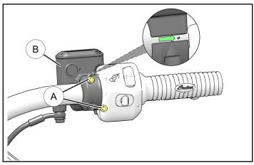
7. Twist throttle fully backward and forward to ensure throttle is properly seated and there is no dragging. If dragging repeat **steps 1 through 6** of this section.
