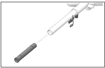
2. Carefully slide accessory handlebar and riser assembly into triple clamp frame. Ensure rubber inserts are installed. Install two retained bolts (B) and washers. Torque to specification. Route handlebar wiring towards front.
