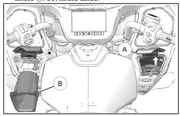
2. Carefully pry along edge with non-marring pry tool to disengage speaker grill assemblies ©.
