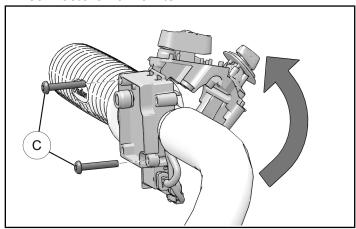
4. Slide RH throttle tube/grip from handlebar.
