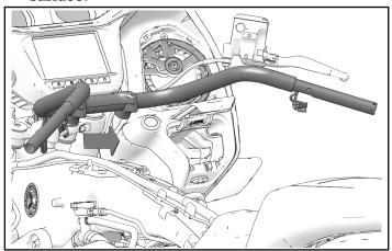
5. Remove and retain weight from LH end of stock handlebar.
