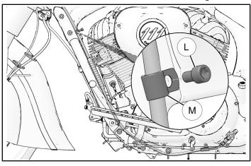
7. Turn handlebars fully right to access cable. Carefully pry cable from wire clip and remove cable.
