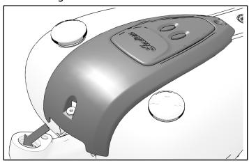
5. Unplug harnesses (switches). Remove back of leather strap from plastic retainer (A) on fuel tank as if removing a shirt button. Remove console from motorcycle and place on a cloth to protect from damage.
