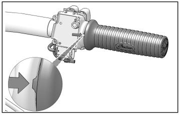
2. Spray three sprays worth of primer into grip opening and allow 5 minutes for primer to dry.
