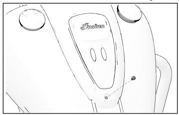
4. Turn handlebars and pull front of console forward to release it from grommet at front mounting location.
