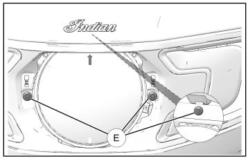
5. Remove and retain two screws (f) from top outer corner of storage openings and two screws (f) from top center of speaker openings.
