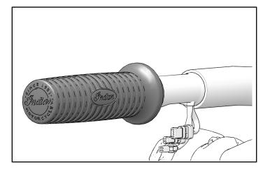
2. Orient throttle housing with pin in rear half of housing and hole in bar as shown. Ensure to line up slots in throttle tube to throttle housing.
