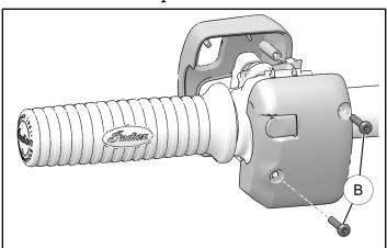
3. Remove and retain two screws © from inner half of RH switch. Rotate switch side upward and remove entire assembly. Disconnect wire connectors from switch.
