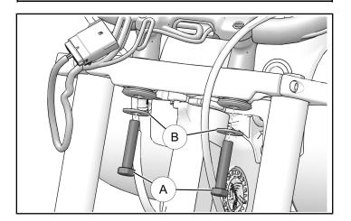
2. Torque rear riser cap screws to specification.
