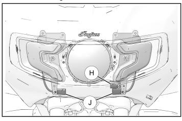
3. Press fairing into place and at top edge to engage locating pins.
