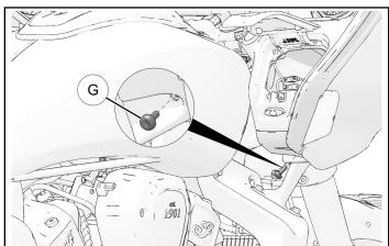
7. Pull fairing outward at top to disengage. Pull fairing out a short distance and disconnect headlight and turn signal wire connectors.
