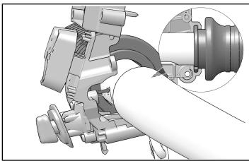
5. Quickly reinstall outer switch assembly with two retained screws ①. Switch assembly notch should fit over tab on grip flange as shown with arrow. Rotate and adjust grip to fit properly. Torque screws to specification.
