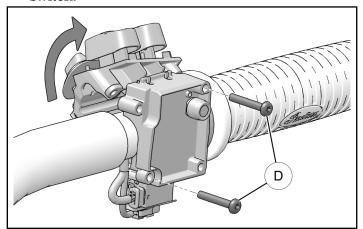
Remove grip by placing rubber strap wrench around LH grip and twisting grip to break adhesive free. Twist grip back and forth while pulling outward. Use a soft hammer if needed to move handle. Discard LH grip.
