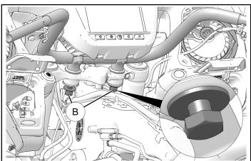
3. Torque rear riser cap screws to specification.
