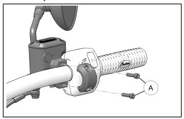
2. Remove and retain two screws (B) from RH switch cube cover and separate halves of cover.
