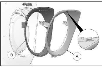
Chieftain® Classic: Install trim piece ® into fairing and secure with two retained screws A. Torque screws to specification.
