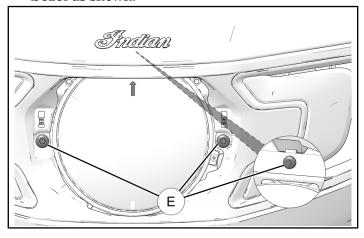
7. Torque all outer fairing screws to specification.
