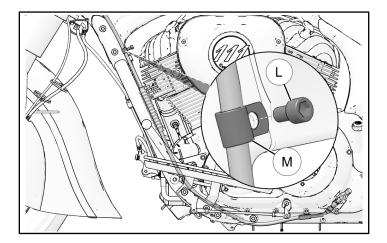
4. Apply multi-purpose grease to lever end of cable barrel and install it in clutch lever at handlebar.
