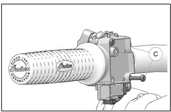
4. Twist throttle fully backward and forward to ensure throttle is properly seated and there is no dragging. If dragging repeat **steps 1 through 3** of this section.
