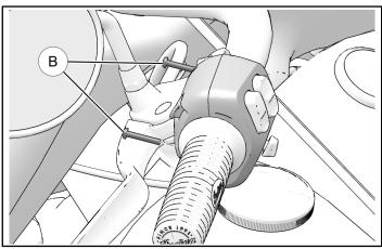
8. Align dimple in handlebar with center of clutch handle assembly halves as shown with arrow. Starting with top screw, torque screws (A) to specification.
