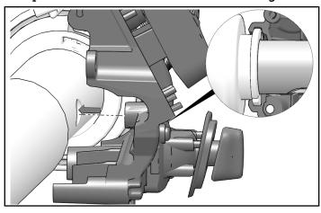
Close throttle housing and reinstall two screws
