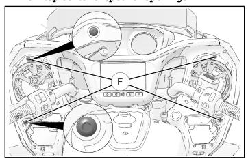
6. Remove and retain one screw © from under edge of each side of fairing as shown.
