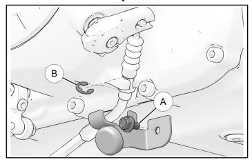
2. Protect clutch release arm © with a shop towel. Rotate release arm inward. Disconnect clutch cable ® from release arm.
