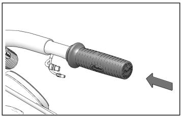
4. Quickly orient switch housing with pin in rear half of housing and hole in bar as shown. Ensure to line up slots on LH Grip to switch housing as shown.
