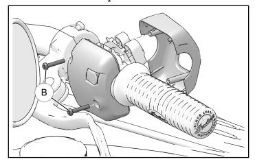
3. Unplug clutch switch connector © from LH switch assembly by using a small pick to release retaining tab. Remove and retain two screws (A) and clutch handle assembly. Remove clutch cable from handle and set clutch handle assembly aside.
