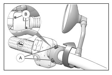
2. Remove and retain two screws (B) from LH switch cube cover and separate halves of cover.
