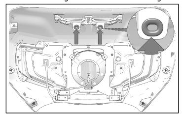
2. Set outer fairing in place and connect turn signal ① and headlight ④ wire connectors.
