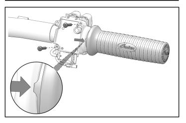
7. Connect all connectors to switch cube assembly and wiring harness as shown.
