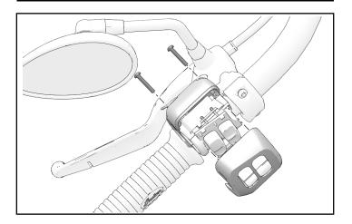
11. Align clutch handle assembly and beginning with top fastener, torque two fasteners to specification.
