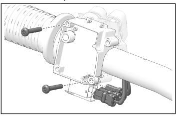
4. Open switch assembly and remove from handlebar.
