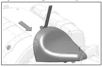
2. Attach driver seat with stud and washer. Torque to specification.
