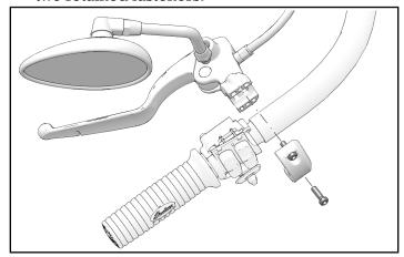
9. Connect clutch wire connector to switch cube assembly.
