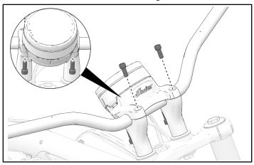
2. Lift instrument housing mount and carefully move out of the way.
