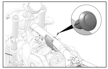
2. Locate harness at opening in center of handlebars and follow to center of bike.
