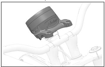
3. Lift and remove handlebar from handlebar mount.
