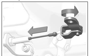
2. Loosen jam nut and remove clutch cable from bracket.
