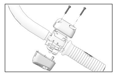
8. Reinstall brake lever assembly using two retained fasteners. Align handle and beginning with top fastener, torque two fasteners to specification.
