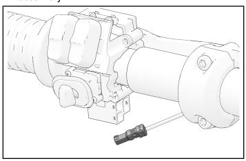
10. Reinstall left-hand switch cube cover using two retained fasteners. Make sure that all wiring is contained within switch cube. Make sure clutch wire is not pinched by two cube covers. Torque fasteners to specification.
