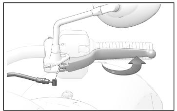
5. Remove clutch cable from wire bracket.
