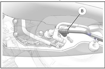
6. Hold tank at front and rear, slide tank upward and rearward to remove.
