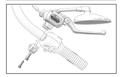
Twist throttle fully backward and forward to make sure throttle is properly seated and there is no dragging. If throttle is dragging, repeat installation.
