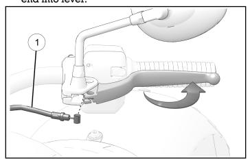
2. Route clutch cable down front of motorcycle and insert into wire bracket.
