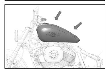
2. Connect fuel vent line ® to fuel tank.
