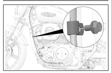
4. Insert clutch cable ① into bracket and thread jam nut onto cable.
