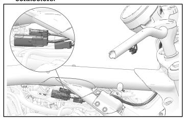
9. Wrap wire harness with cloth and attach with retained push-pin rivet.
