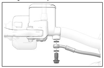
2. Follow brake hose to brake manifold. Remove pressure switch, washers, and brake line from manifold.
