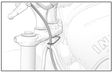
3. Install clip and attach with retained screw. Torque screw to specification.
