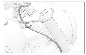
3. Install new brake hose ② and two new crush washers ④ to master cylinder. Make sure brake hose is routed properly and torque both upper and lower brake hose banjo bolts to specification.
