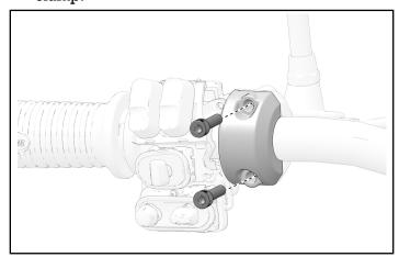
6. Remove perch clamp and clutch lever.
