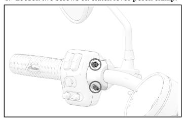
2. Carefully rotate clutch lever until both screws on switch cube can be accessed.
