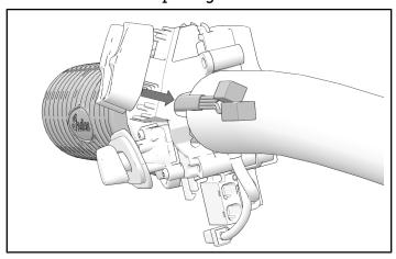
Quickly attach inner switch cube with two retained fasteners. Switch cube assembly notch should fit over tab on grip flange as shown with arrow. Rotate and adjust grip to fit properly.
