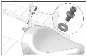
4. Remove the driver's seat by lifting up on the seat bracket and pulling the seat rearward.
