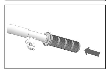
4. Quickly orient inner switch cube so pin is inserted into handlebar. Make sure to line up slots on left-hand grip to inner switch cube, as shown.
