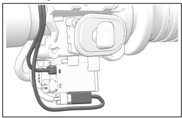
Reinstall right-hand switch cube cover using two retained screws. Make sure that all wiring is contained within switch cube. Torque fasteners to specification.
