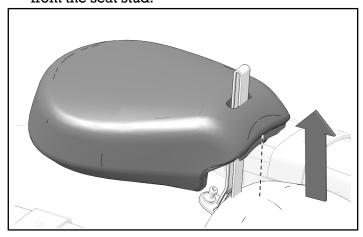
3. Remove the seat stud and washer from the strap bracket.
