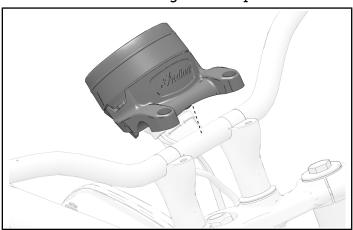
6. Install four handlebar clamp fasteners and torque to specification. Torque front fasteners first, then rear fasteners.
