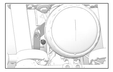
6. Attach bracket with retained screw to left hand front isolator and torque to specification.
