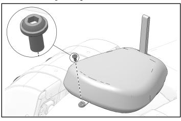
2. Remove the passenger seat by lifting up on the front edge of the seat to disengage the grommet from the seat stud.
