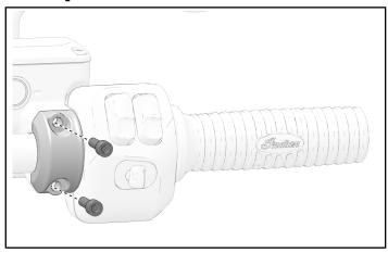
2. Remove perch clamp and brake lever.
