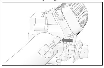
4. Close inner switch cube and reinstall two inner cube fasteners. Torque fasteners to specification.
