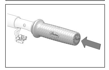
2. Orient inner switch cube so pin is inserted into handlebar. Make sure to line up slots in throttle tube to inner switch cube.
