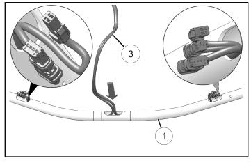
2. Pull right hand harness through until Electronic Throttle Control (ETC) connector **8F** is visible in opening and pull connector out of opening.
