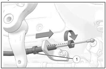
5. Rotate pinion arm and install clutch cable ① into arm
