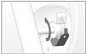
5. Attach bracket with retained screw to right hand front isolator and torque to specification.
