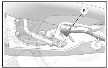
3. Connect fuel pump electrical connector (A).
