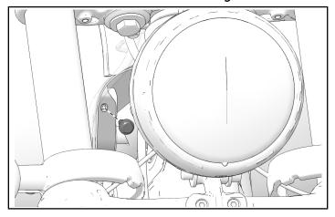
3. Rotate both fuel tank brackets downward to disconnect from isolator.
