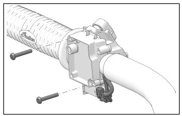
Twist throttle fully backward and forward to make sure throttle is properly seated and there is no dragging. If throttle is dragging, repeat previous two steps. 6. Connect all connectors to switch cube assembly and wiring harness as shown.
