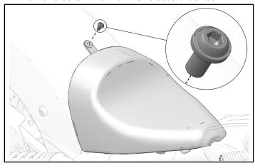
2. Lift up on the seat bracket and pull the seat rearward to remove.
