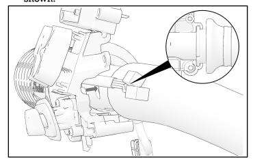
5. When inner switch cube is closed, heated grip wire should exit opening shown with arrow.
