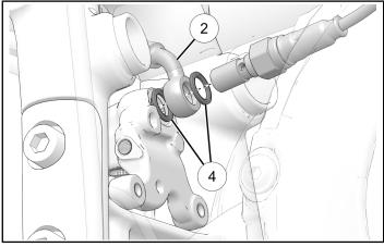
2. Route brake hose up toward right handlebar grip. Install brake hose into metal wire bracket.
