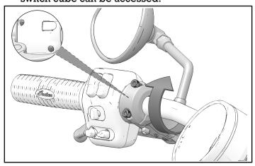
3. Remove two screws and switch cube halves.
