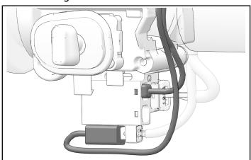
8. Loosely reinstall clutch lever assembly using two retained fasteners.
