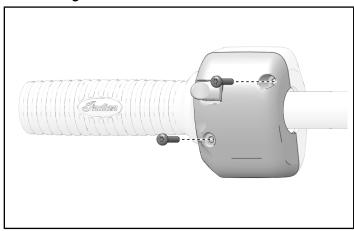
2. Remove switch cube outer housing halves.
