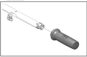
2. Disconnect electronic throttle control (ETC) from handlebar harness and remove ETC from handlebar.
