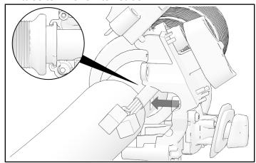
3. When inner switch cube is closed, heated grip wire should exit opening shown with arrow.
