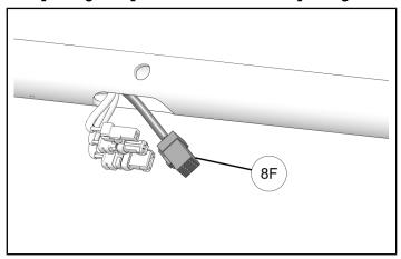
3. Install ETC into handlebar end and connect to **8F** connector.
