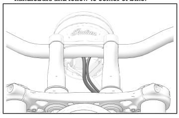
3. Disconnect three connectors from handlebar harness in center of frame.
