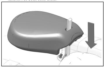
4. Attach passenger seat with screw. Torque screw to specification.
