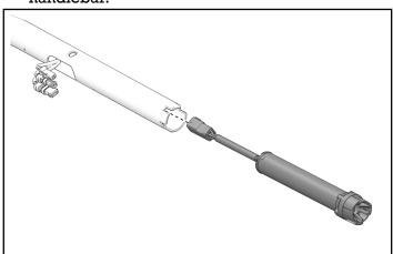
Install rubber strap wrench around left hand grip and twist grip to break adhesive free. Use caution to not damage grip. Twist grip back and forth while pulling outward to remove.
