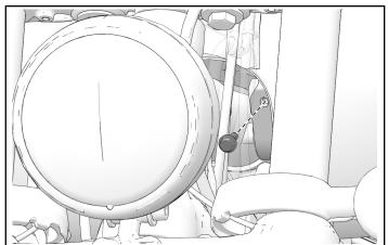
2. Remove screw from bracket under right hand front of tank and let bracket hang.
