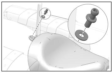
3. Pull strap through opening in passenger seat and lower seat onto stud.
