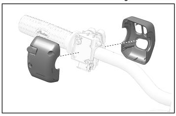
3. Remove three connectors and two screws from switch assembly.
