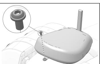
2. Attach driver seat with screw. Torque to specification.
