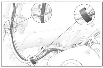
8. Connect handle bar harness to chassis connectors.
