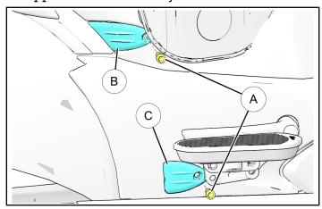
2. Install RH highway bar ② using three new screws ③. Torque screws to specification.
