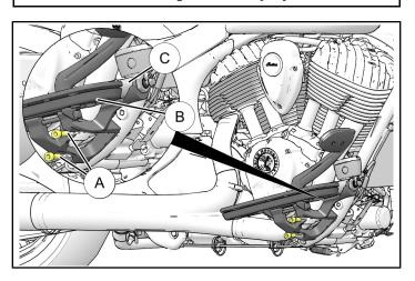
2. Remove and retain two screws (A) from left hand foot control assembly (D).
