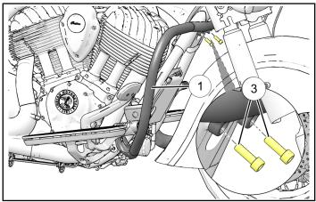
2. Loosely install side mounts of front highway bar
