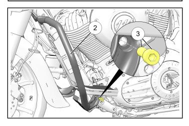
3. Hold RH highway bar ① in place and loosely install screw ③ as shown. **DO NOT** torque fastener at this time.
