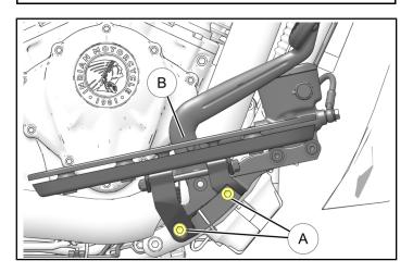
2. Hold LH highway bar (2) in place and loosely install screw (3) as shown. **DO NOT** torque fastener at this time.
