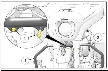
5. Align LH (2) and RH (1) highway bars and torque lower fasteners (3) to specification.
