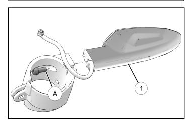
2. Ensure turn signal ① harness routes within channel of turn signal mount.
