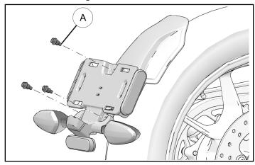
Pinch two tabs on license plate mount to disassemble from debris shield. Harnesses will need to be routed out of debris shield opening during disassembly.
