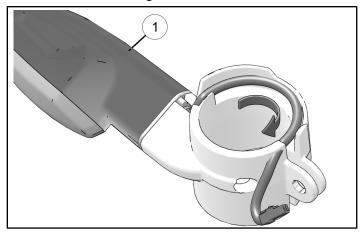
3. Install turn signal mount onto suspension fork with one retained screw (B) and one retained washer (C).
