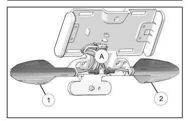
Route turn signal and license plate harnesses through debris shield opening before replacing license plate mount onto debris shield. Ensure two license plate mounts full engage within debris shield.
