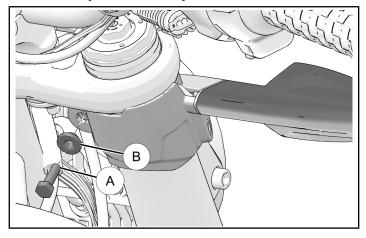
3. Remove and retain one screw © from within turn signal mount to uninstall stock turn signal. Discard stock turn signal.
