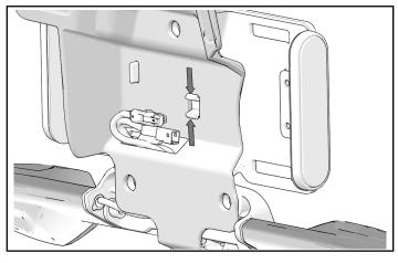
5. Remove and retain two screws from each turn signal.
