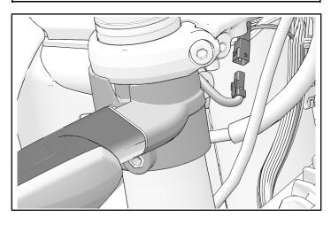
2. Remove and retain one screw (A) and one washer (B) from turn signal mount. Remove turn signal assembly from motorcycle.
