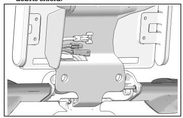
3. Reinstall license plate assembly onto license plate arm with three screws **B**.
