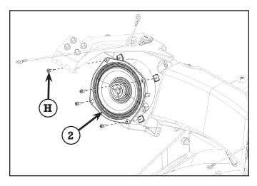
13. Replace speaker grilles and lower trunk pad. Torque fasteners to 36 in-lbs. (4.06 Nm).
