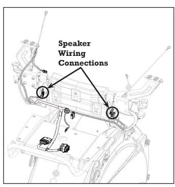
12. Attach RH side speakers (2) using screws (H) from speaker plates. Torque to 18 in-lbs (2.03 Nm). Repeat the same for LH side also. Connect the speaker with wiring connector.
