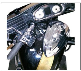
10. Before fully removing the console, disconnect the three wire harness connectors (D) (power button, bag lock, and heated grips (if installed)). Mark the connectors with a marker before unplugging to aid in identification for re-assembly.
