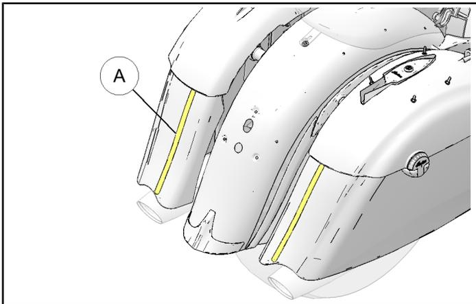
2. Ensure residue is removed from bag before installation of new trim.
