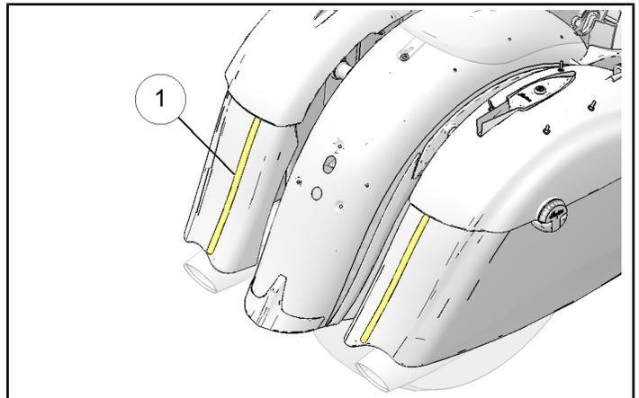
5. Apply firm pressure along the trim during installation. Confirm all edges are adhered to the saddlebag.
