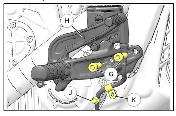
5. Loosely install extended reach mount ② using retained screws ⑥ (removed in previous step). Install front screw only finger-tight. Install rear screw and torque **only rear screw** to specification. Remove front screw and retain for next step.
