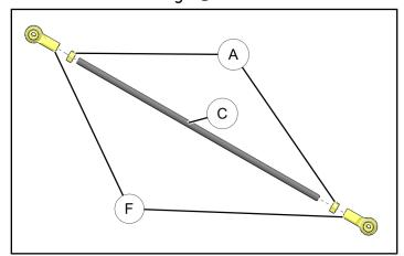
7. Install jam nuts (A) and rod ends (F) onto new shift linkage (4). Adjust spacing between center of openings in rod ends to 406 mm (16 in.) by turning both rod ends evenly onto shift rod.
