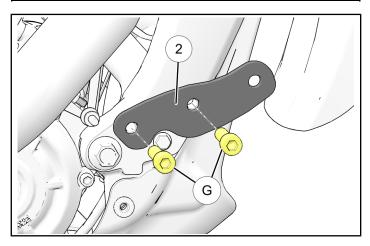
6. Align holes in RH foot control (H) and install to extended reach bracket (2) using retained screw
