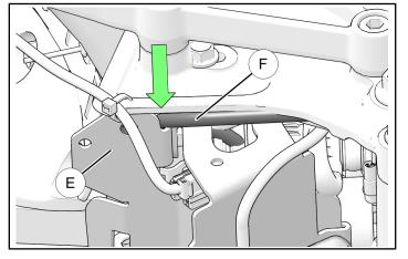
c. Pull all slack from brake line starting from ABS module forward to brake pedal master cylinder. d. Reinstall retained screw © and torque both screws © and D to specification.
