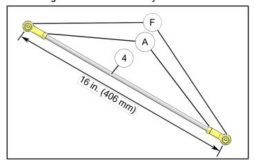
8. Install new shift linkage 4 using two new screws
