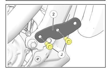
7. Align holes in RH foot control (®) and install to extended reach bracket (2) using retained screw (1) and new screw (7) and nut (9). Torque fasteners to specification.
