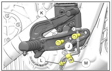
6. Loosely install extended reach mount ② using retained screws ① (removed in previous step). Install front screw only finger-tight. Install rear screw and torque **only rear screw** to specification. Remove front screw and retain for next step.
