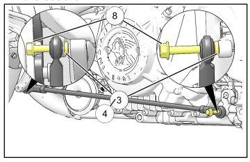
9. Set desired shifter lever position by threading shift rod in or out of rod ends. Torque jam nuts (A) on shifter linkage (4) to specification.
