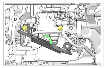
b. Move brake line **(F)** from routing behind bracket **(E)** to route through gap on front side of bracket as shown.
