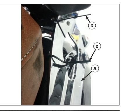
6. Route harness (1) through wire retainer and connect harness to trunk connector (B) and place as shown in figure.
