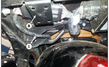
**CAUTION:** Contact between the harness and painted surfaces will cause paint damage. Ensure that the harness is fastened properly and securely and there is no contact possible before riding the motorcycle.
