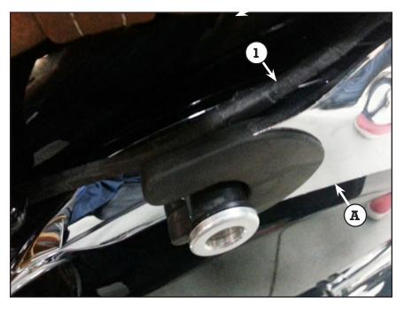
5. Using panduits (2), attach the harness to trunk frame (A) as shown in figures. Be sure to tie harness in such a manner as to prevent contact with painted surfaces.
