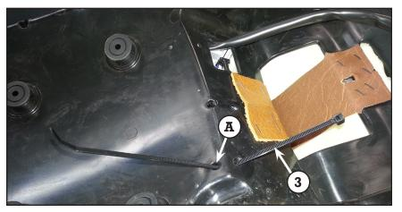
Place harness (1) on seat base. Align the white tape (B) with the panduit (3). Short side of harness (1) should go to the center of the seat. Tighten panduit (3) and cut off excess.
