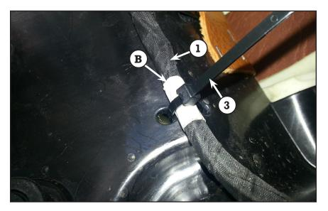
5. Press the harness (1) into clips in seat base.
