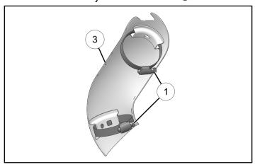
2. Open the worm-drive clamps far enough to slip them over the exhaust pipe, and then put the accessory rear heat shield ③ on the motorcycle.
