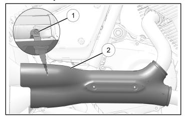
3. Install the two heat shield fasteners (£) and torque to specification.
