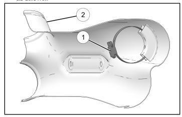
2. Open the worm-drive clamp far enough to slip it over the exhaust pipe, and then put the accessory catalytic converter heat shield ② on the motorcycle.
