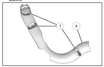
2. Open the worm-drive clamps far enough to slip them over the exhaust pipe, and then put the accessory front heat shield ④ on the motorcycle. Make sure the clamps are set as shown.
