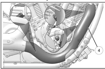
3. Make sure the seams between the heat shields are aligned, and then torque the worm-drive clamps to specification.
