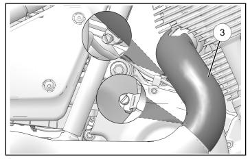
3. Make sure the seams between the heat shields are aligned, and then torque the worm-drive clamps to specification.
