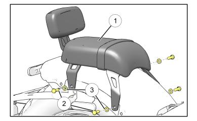
7. Remove rubber blanks ① from each strut cover.
