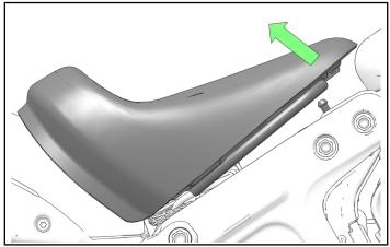
2. Lift front of seat and slide forward to disengage seat base tabs from rear fender and carefully set seat aside.
