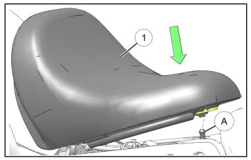
3. Pull up on seat to ensure it is firmly attached.
