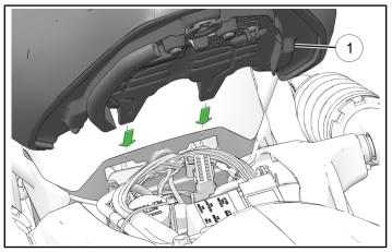
2. Align seat grommet with pin (A) and press firmly down on seat to lock in place.
