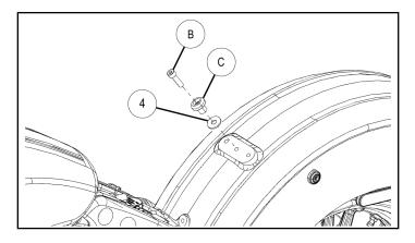
2. If passenger seat or solo rack is not installed: Place backrest bracket ① onto motorcycle as shown with two large washers ④ between the fender frame and backrest bracket. Install two M8 hex head screws ② in the holes by the seat mounting post and torque to specification.
