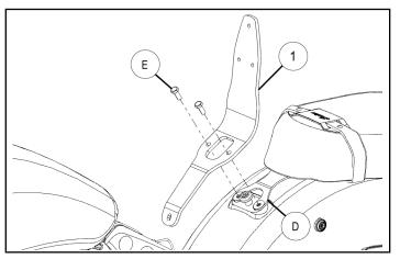
3. Install one M8 Screw ② and one small washer ③ to secure the front side of the bracket and torque to specification.
