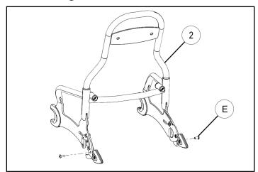
5. Place front mounts (F) of backrest onto front spool bushing assembly. Rotate passenger backrest down onto vehicle and lock into place by rotating lock levers downwards as shown.
