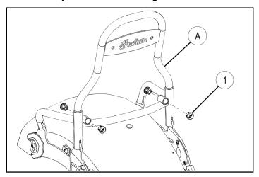
2. Ensure all front and rear plugs ① fitted properly to the sleeves.
