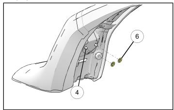
7. Place your sport seat ① on the bike and start to thread the sport seat logo screws ④ into the frame to help align the seat. At this point do not fully tighten the screws.
