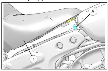
9. Secure the rear potion of the seat ① to the fender using screw ⑤ and washers ⑥ ⑦. Torque the sport seat logo screws ④ and then rear screw ⑤ to specification.
