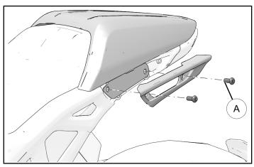
5. Adjust seat cowl height to ensure even spacing along sub-frame and rear light.
