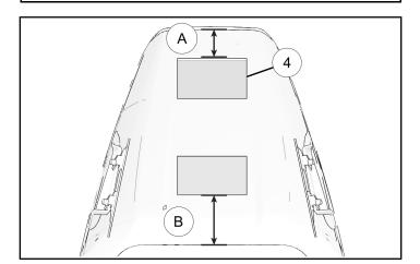
4. Place seat cowl assembly over rear portion of seat and pass retained fasteners (4) through passenger handles and seat cowl brackets.
