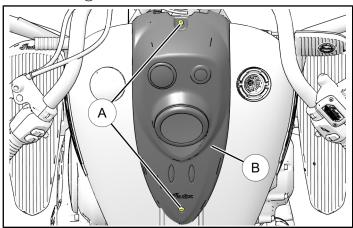
2. Carefully lift tank console ® from tank, reach under console an unplug any connectors that may be installed. Carefully set tank console ® on a cloth to protect finish.
