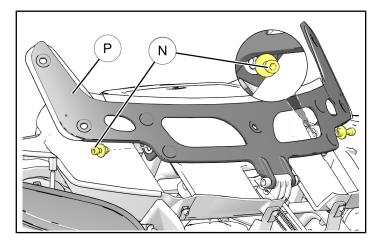
6. Install outer fairing. Install six retained screws in original locations. Torque screws to specification.
