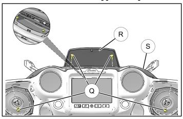
c. Pull rubber weather strip ① from edge of upper dash piece ③. Push upper dash piece ⑤ forward until tabs are clear of inner fairing (shown with arrows) and lift upper dash piece ⑤ up and out around windshield bracket P and set aside.
