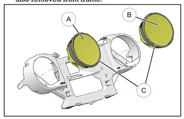
2. Install new speedometer ① in left hand opening and new tachometer ② in right hand opening with pre-installed grommets ⑤ into gauge frame. Align holes in frame with holes in gauges as shown.
