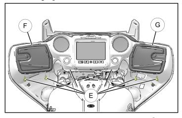
d. Remove and retain six fasteners  $\mbox{$\mathbb{H}$}$  from inner fairing assembly.
