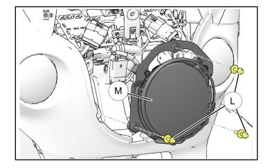
8. Install head light bezel (with two retained screws (). Torque screws to specification.
