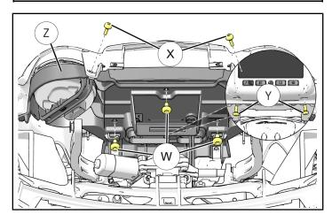
5. Pull rear gauge frame ② forward and up to remove from front fairing and set aside. Leave touchscreen display installed in fairing.
