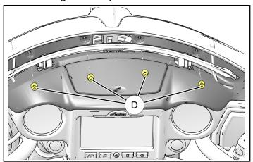
c. Remove and retain 4 screws ©. Remove and retain left © and right © speaker grills by using a plastic trim removal tool.
