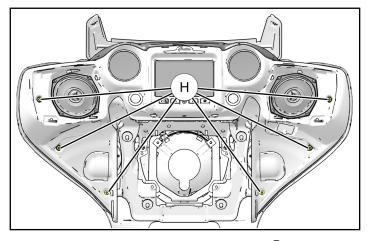
e. Remove and retain two screws  $\bigcirc$  from head light bezel  $\bigcirc$ . Pull firmly outward to remove head light bezel  $\bigcirc$ .
