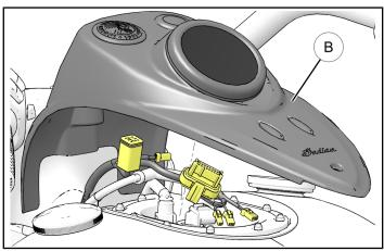
3. Set tank console (B) face down on soft cloth and remove and retain two inner screws (C), two outer screws (D), and gauge bracket (E).
