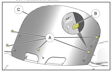
b. Remove and retain four screws (1) from top of fairing assembly.
