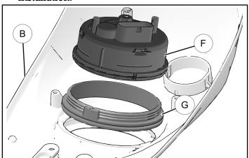
5. Transfer retained grommet © to new gauge ①. Install new gauge assembly into tank console ®.
