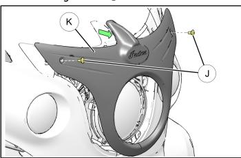
f. Remove and retain three fasteners ① and withdraw head light assembly ⑩ far enough to disconnect electrical connector. Remove head light assembly and set aside.
