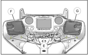
10. Install four retained screws ① in top of fairing assembly. Torque screws to specification.
