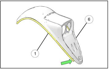
Install switches/blanks (#) (removed in Step 6 of Removal section) to new console (6). Use four new screws (4) and torque to specification.
