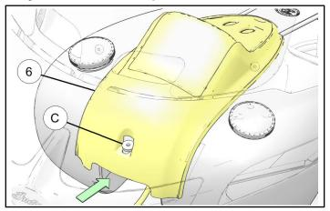
12. Install new rear mounting screw (5). Adjust console front to rear to align screw hole. Torque screw to specification.
