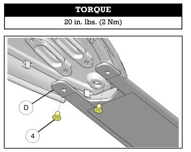
10. Being careful not to damage paint on fuel tank, set console onto tank. Ensure console harness, fuel line and vent lines are routed out of front of console without being pinched.
