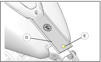
5. Remove two screws (F) and remove leather tank strap (D) from back of console.
