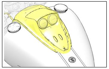
11. Push console (6) rearward onto front mounting grommet (C) until fully seated.
