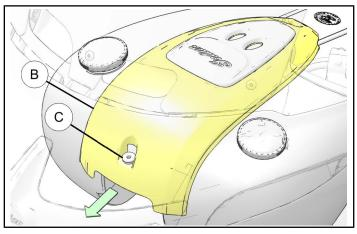
4. Unplug harnesses (switches). Remove back of leather strap () from plastic retainer (E) on fuel tank as if removing a shirt button. Remove console from motorcycle and place on a cloth to protect from damage.
