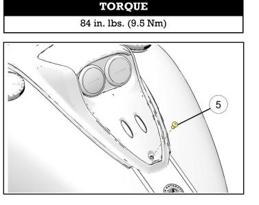
13. Fasten tank strap (D), (removed in **Step 4** in **Removal** section), to plastic retainer at rear of fuel tank. Pull leather strap over plastic retainer as if buttoning a shirt. If plastic retainer was damaged, remove old part completely from hole, and use new clip (2).
