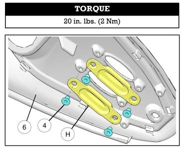
3. Install lower applique ① from kit PN 2881847-XX onto console ⑥. Tabs on applique fit into slots on console. Ensure openings for switches are properly aligned and bend tabs of applique outward onto backside of console.
