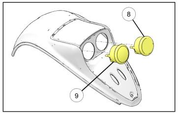
5. Use new brackets (1) and nuts (3) to secure gauges from backside of console. Torque nuts to specification.
