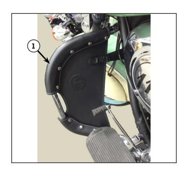
2. Connect the straps (B). The straps can either be connected to the clip on the opposite closeout, or to the frame (A). See figures. Tighten the straps until they are snug.
