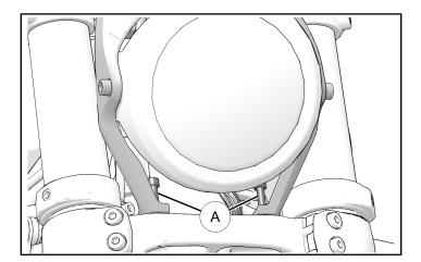
7. Ensure two screws (10) pass through spacers and reinstall headlight bracket. Torque two bracket fasteners (9) during this step.
