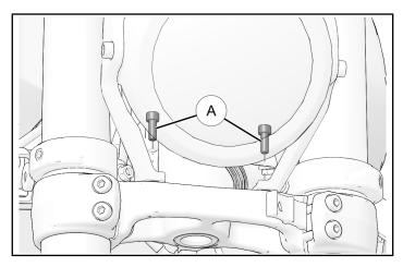
3. With headlight assembly unmounted, tilt assembly forward and slide electronic throttle control (ETC) connection off push-pin clip. It is not necessary to disconnect harnesses.
