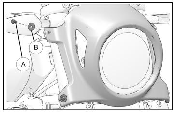
2. Remove headlight cowl and set aside for reinstallation.
