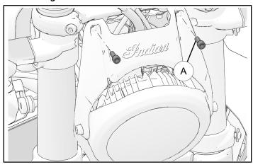
2. Remove and retain two screws (A) from bottom of headlight bracket.
