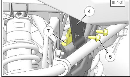
Install link mount (item 3) to main bracket (item #4) using four bolts (item #5). (See illustration 1-3). Tighten M8 hardware to specification.
