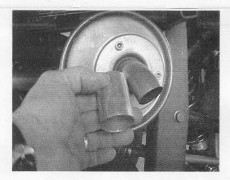
Cut outlet at angle to allow 1 3/8" weld on adapter to be welded on at downward angle.
