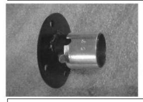
To use elbow adapter, slide #59 bushing onto the outlet as shown. This make it 1 ½" O.D. needed for use with elbow. Use sealant.
