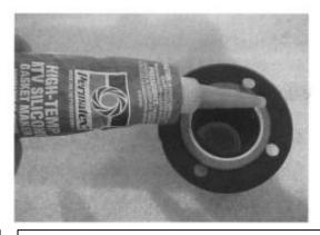
Glue gasket in place with HI-TEMP silicone and apply silicone to all surfaces and screw holes
