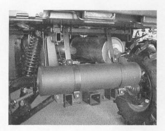
Assemble hangers to muufler and mount as shown by drilling holes in crossmember.
