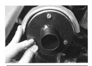
Install Adapter-Tighten Bolts Evenly- Let Silicone Dry- Recheck Bolts After Running
