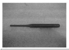
Enlarge holes with 3/16" pin punch such as one shown. This rolls metal inside to make screws grip better.
