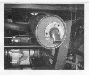
Or remove spark arrester and drill new holes so it points down instead of to the right.
