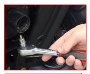
Remove the existing hex bolt from the OEM muffler as shown.
