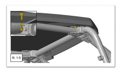
Loosely install the M6 x 45mm Torx Screws (Item #2), Oversize Washer (Item #4) and Flanged Lock Nut (Item #5) on two front mounting holes. Be sure not to cross thread fasteners. (See Illustration 1-6).
