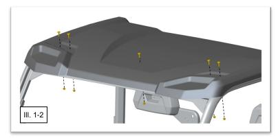
Loosely install the four M6 x 25mm Torx Screws (Item #2) and Nylon Spacers (Item #3) in the rear mounting holes. The Nylon Spacers go between the Poly Roof and the Roll Cage. The Torx Screws will self tap threads into the OEM holes in the roll cage. (See Illustration 1-3).
