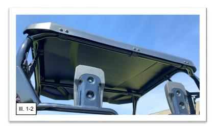
Insert Rubber Spacer (Item #3) into each Clamp. Then loosely install a Lock Washer (Item #5) and Button Head Hex Screw (Item #6) into each Clamp to hold it closed. The two remaining Rubber Spacers can be discarded. (See Illustration 1-3).
