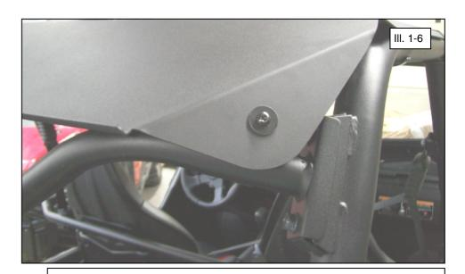
Continue to attach the larger clamps (item #9) around the cab frame at each of the slotted hole locations. Fasten using M6 screws (item #3) and flat washers (item #5) through the top surface. Secure clamps into position from lower surface with M6 locknuts (item #4) as shown. (See illustrations 1-7, 1-8 and 1-9).
